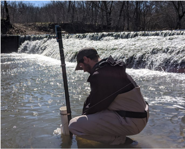
Justin Brisendine installs aquatic water quality sensors on McDiffit Creek, Kansas to assess biological and physical conditions in the stream that could influence aquatic microbiomes.
